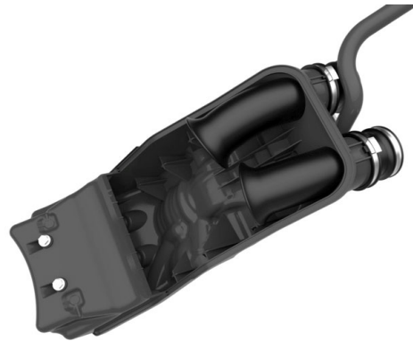
Air Cleaner Box (inside)
