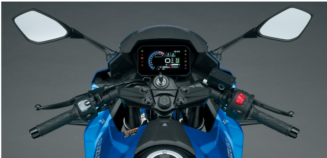
Forged Aluminum Separate Handlebars
